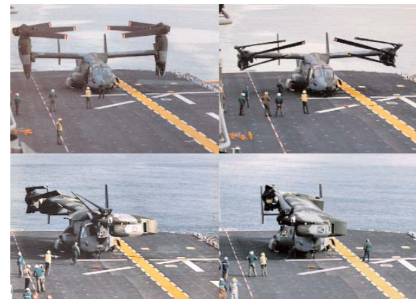
Blade Fold/Wing Stow Sequence
